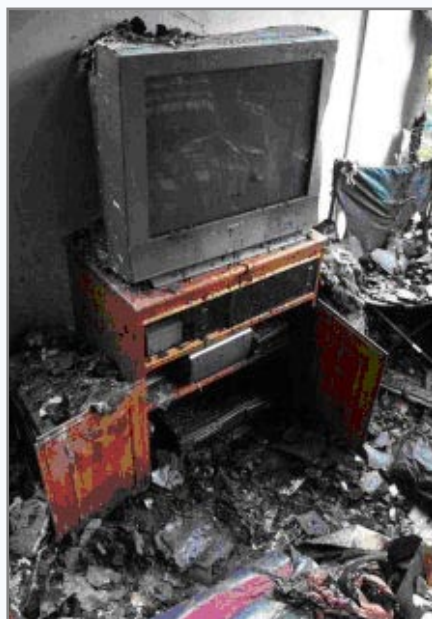
A TV set that was saved from fire since it had Hexabromobiphenyl in it.
